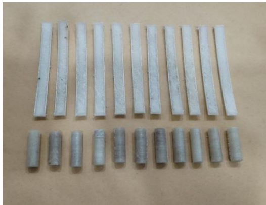
0.3% Kenaf-reinforced nylon specimens
