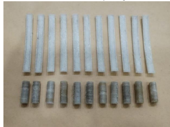
0.5% Kenaf-reinforced nylon specimens
