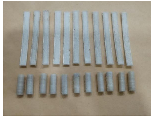
0.1% Kenaf-reinforced nylon specimens
