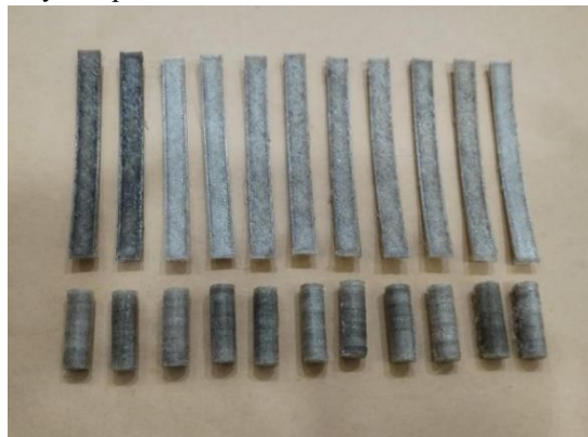
1% Kenaf-reinforced nylon specimens
